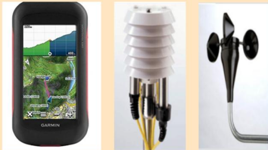
GPS, Metrological Humidity Temp. Probes, Wind speed sensors funded by Sathyabama
